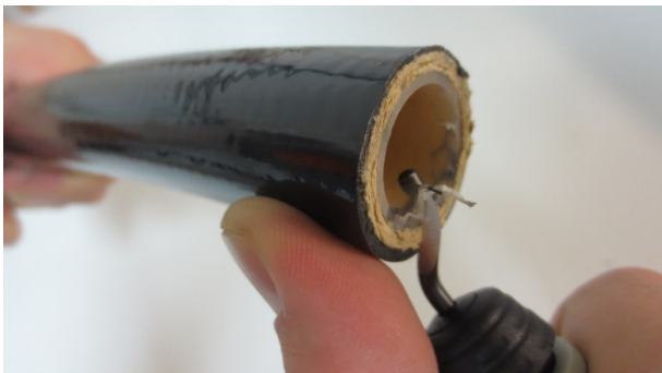
Use a proper tool to remove burrs and/or residual from the cut surface.
