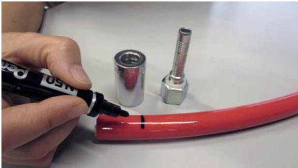
Marking the insertion depth of the ferrule and then put insert into the hose.
